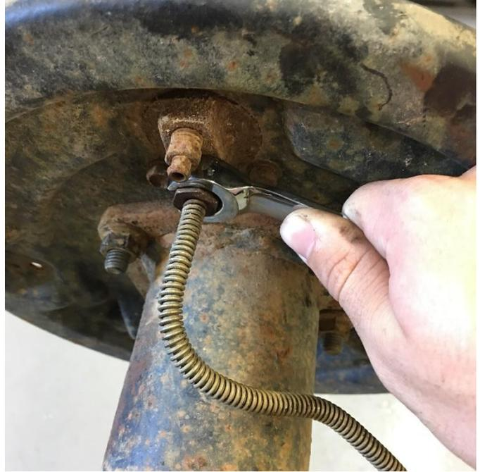
The cable can then be removed from the backing plate by depressing its perimeter springs. Remove the brake line from the wheel cylinder using a line wrench if possible.
