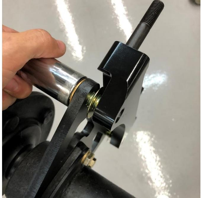
Bolt on the brackets using the supplied hardware, as shown. The calipers should be mounted to the **REAR** of the axle. The radial brackets can temporarily be installed at this time using the supplied M14 bolts and washers, along with two .563x1.125x.035 shim washers between the axle bracket and radial bracket. If you have the optional braided hose kit, the hose bracket will also be installed at this time as shown using the provided hardware.
