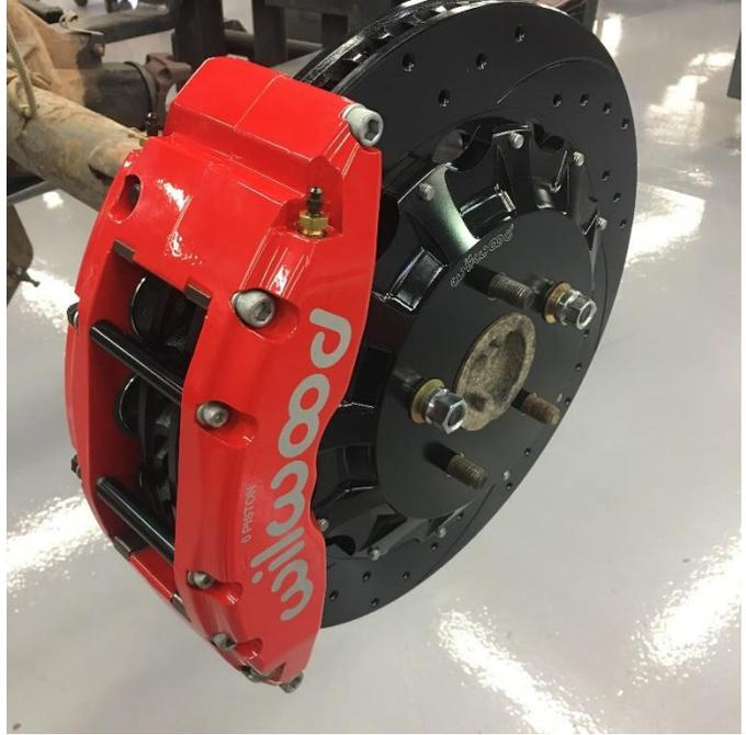
If you do not plan on installing new brake lines, the factory brake line can then be rerouted and tightened into the stainless hose. It is best to use a wrench to support the stainless hose from spinning in the hose bracket.
